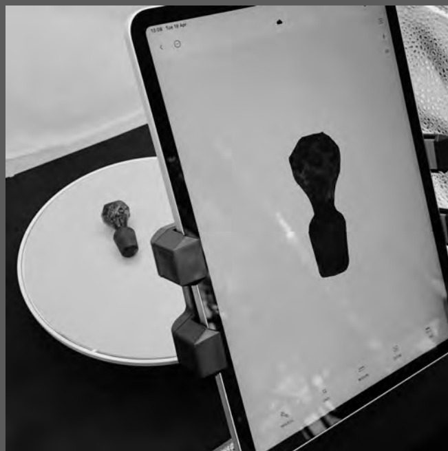
THE IPAD SET UP ON A STEADY STAND WITH THE OBJECT ON A TURNTABLE.
